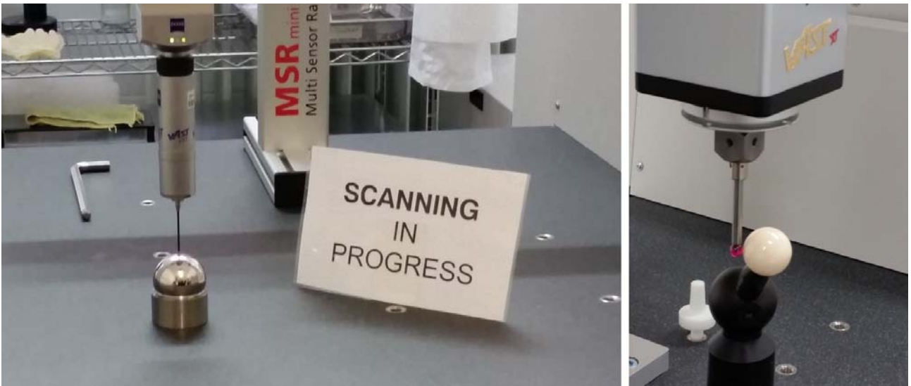
Figure 1: surface scanning of surface of metal (left) and ceramic (right) hip implants at the London Implant Retrieval Centre
