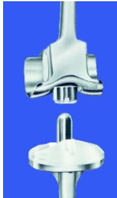
Figure 8. A linked prosthesis (Rotalink) without patellar flange. The femoral housing contains a PE lined hinge. The tibial metal protrusion articulates against a PE lined tube connected to the hinge thus allowing axial rotation.
